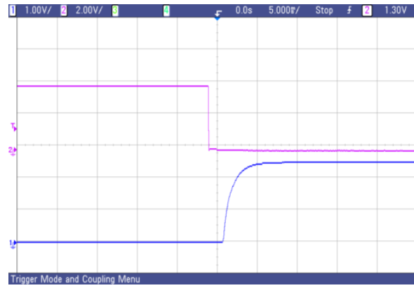
Fig. 64 AVO75-48S2V5 typical start-up from CNT on
