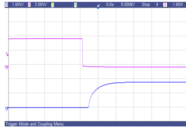
Fig. 62 AVO75-48S1V8 typical start-up from CNT on
