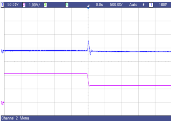
Fig. 30 AVO75-48S1V8 typical transient response to step decrease in load from 50% to 25% of full load, room temperature, 48Vdc input ( \Delta I_o/\Delta t=0.1A/1\mu s )
