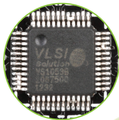
Figure 8-1: On-board VS1053 MP3 codec
