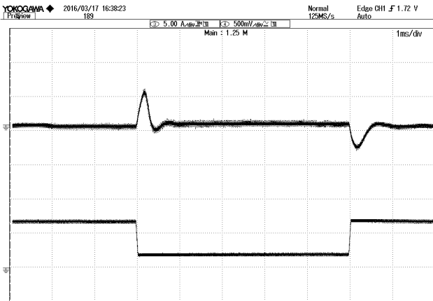
Figure 4: Dynamic response to load step 25%~75% with 0.1A/uS slew rate at 110/220Vac\ TOP:Vout,500mV/div, BOTTOM:Iout,5A/div, 1mS/div
